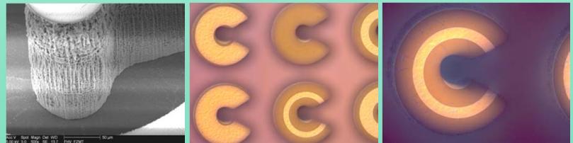
Fig. 4. Detail of the patterned 330 μm high Si-pillar. Fig. 5. Back-side view of patterned ring membrane based C-HEMT sensor arrays. Fig. 6. Detail of C-HEMT sensor from the back-side.
